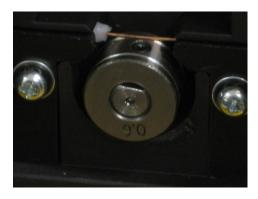
Feed the loose end of the wire through the Inlet Guide Tube, past the drive roll and into the back of the MIG Gun. Keep tension on the wire to prevent unspooling on the spool. Make certain wire is centered on groove and adjust drive roll (Step 3) if needed.
