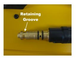
This MIG gun is a one piece connection. Notice the retaining groove on the machine end. The hex-headed retaining screw in the step (6) will set down into this groove.
