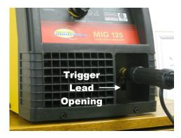
Remove Retaining Screw (see step 6) Slide the machine end of the MIG gun into the front panel receptacle. Push it all the way into the wire feeder as far as it will go. Feed trigger leads through the opening in the front panel. 6
