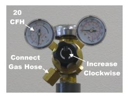
Open the drive roll tension arm on the wire feeder. Open the valve on the shielding gas bottle. Turn on the unit power and pull the trigger. Adjust the regulator to set for 20 cubic feet per minute. Reinstall the drive roll tension arm on the wire feeder.
