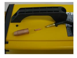
To finish feeding the wire through the MIG gun, you will need to remove the gun nozzle and tip.
