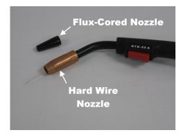
Slide the correct size contact tip for the wire size you are using over the end of the wire and tighten clockwise to secure. Choose the correct nozzle, thread on nozzle and clip any excess wire.
