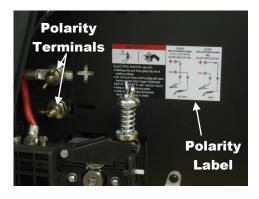
Feed ground cable through the front opening. Install on the open polarity terminal. Solid wire uses Electrode Positive (DCEP) polarity. Flux-cored wire use Electrode Negative (DCEN) polarity. See polarity label in the wire compartment and change as needed.
