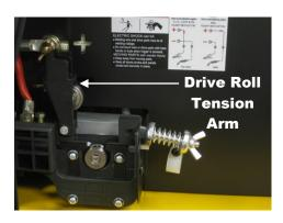
Open the drive roll tension arm on the wire feeder.
