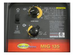
On the wire compartment access panel is a set-up guide. Find the type of material being welded and the size of wire you are using. Slide over to the thickness of the thinnest material you are welding. Set the voltage and wire feed speed on the front of the unit.
