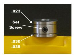
The smaller groove on the drive roll is to be used with .023 wire. The larger groove can be used for .030 and .035 wire. Use the supplied "L" shaped hex wrench to loosen set screw and to align the proper groove to the wire path. Retighten set screw.
