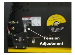
Close the drive roll tension arm. Apply tension to the wire by turning the wing nut clockwise on the Drive Roll Tension Adjustment. Do not overtighten. See Step 14.
