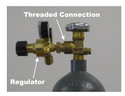
Thread the regulator directly to the bottle. A CO2 adapter will be needed if using straight CO2 gas. One end of the supplied gas hose connects to the regulator. The other end connects to the gas valve on the back of the machine.
