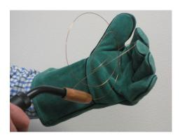
Test drive roll tension by feeding wire into a gloved hand from about 4 inches away. Loosen tension to apply little pressure. Slowly increase tension until the wire coils up in your hand without slipping in the drive rolls.
