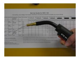
Stretch out the MIG gun. Turn on input power and pull the trigger to feed the wire through the gun. Stop when the wire pushes through the end of the gun.
