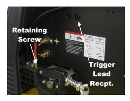
Tighten the retaining screw on the wire feeder housing to secure the gun. Install trigger leads into the trigger lead receptacle.
