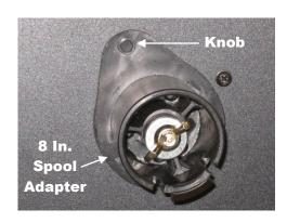
Remove wing nut, washer and black bushing. Slide on spool adapter. Reinstall bushing, washer and wing nut. Slide on 8" spool of wire. Knob on spool adapter slides into hole on side of 8" spool of wire. See Step 13 to adjust wire spool tension.
