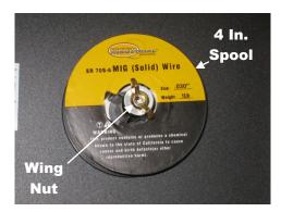
Remove wing nut, washer and black bushing. Slide on spool so wire feeds off the bottom of spool. Reinstall bushing, washer and wing nut. See Step 13 to adjust wire spool tension.
