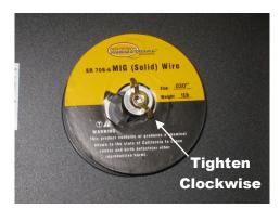
Adjust the wing nut in the center of the spool to adjust spool tension. A small amount of slack should be in the weld wire when wire feeding stops. Too much tension will cause poor feeding. Too little tension will cause the wire on the spool to uncoil.
