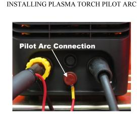
Remove the red thumb screw and the flat washer on the front of the machine. Install the red lead with the round terminal onto the pilot arc terminal. Reinstall the washer and tighten the thumb screw.
