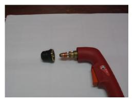
The nozzle sets on top of the electrode.
