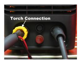
Install the machine end of the plasma torch to the negative (-) receptacle on the front of the machine.
