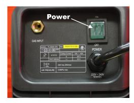
Install input power to the proper receptacle and turn on the unit power using the power switch on the back of the unit.
