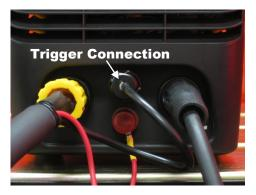
Line up the key way in the trigger receptacle with the key way on the trigger plug on the black trigger lead. Push to install. Listen for the snap.
