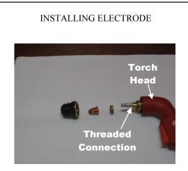
The electrode is threaded into the torch head. Install by turning clockwise.
