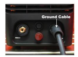
This unit requires a completed electrical circuit in order to operate correctly. The ground cable and clamp completes the circuit. Connect the ground cable to the positive (+) receptacle on the front of the machine.
