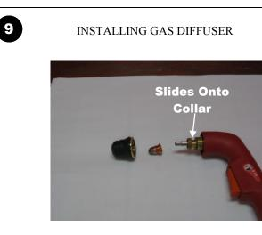
The gas diffuser slides over the electrode and connects to torch head.
