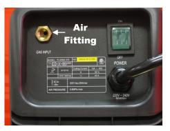
This unit requires compressed air to operate. You can use an air compressor or a bottle of compressed air. The air supply to the bottle should be at least 70 PSI. Make the connection to gas fitting on the back of your unit.
