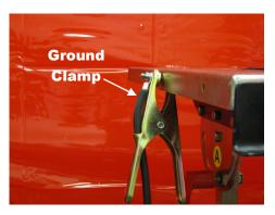
It is important that the ground clamp is properly secured to a clean, paint free connection either on the cutting table or the work piece.
