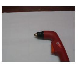
The torch cover threads onto the torch head. Install by applying slight inward pressure and turning clockwise. Hand tighten.
