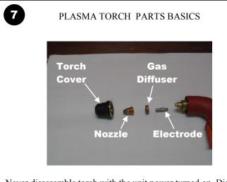
Never disassemble torch with the unit power turned on. Disconnect input power before proceeding. This torch has four replacement parts. Remove torch cover by turning counter clockwise. Nozzle sets atop electrode. Gas diffuser sets on the torch head.
